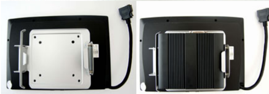
Example : QBOX mounted on CTF840-SH TFT display
